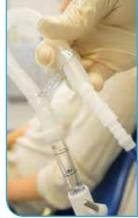
**Vacuum control** block, vacuum hose with a hanger and an adapter
